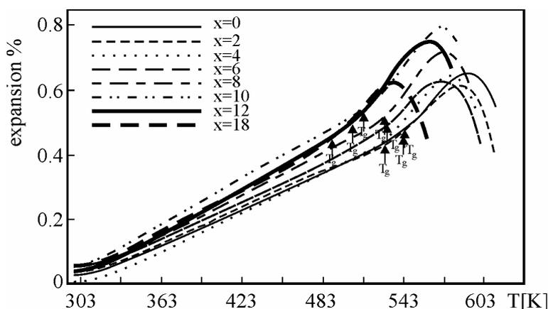
Fig. 12. DTD curves of the glasses  $\text{Ge}_{20}\text{As}_{14}(\text{S}_{0.5}\text{Se}_{0.5})_{66-x}\text{I}_x$ .
