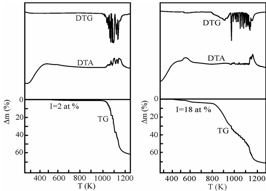
Fig. 8. DTG, TG and DTA curves for  $Ge_{20}As_{14}(S_{0.5}Se_{0.5})_{66-x}I_x$ .
