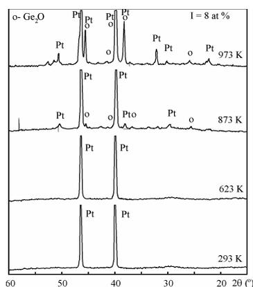
Fig. 11. High-temperature diffractogram of the glass  $\text{Ge}_{20}\text{As}_{14}\text{S}_{29}\text{Se}_{29}\text{I}_8$ .
